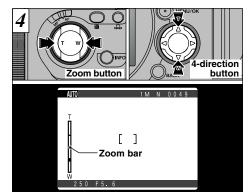
You can use the Zoom button or "▲" and "▼" on the 4-direction button to zoom in and out. To zoom in on the subject, press the T side of the button. To zoom out, press the W side. When you use the zoom, a "zoom bar" appears on the screen.
